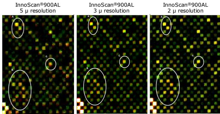
Figure 3a. Examples of **1x385K (16  $\mu$  spot size)** Roche NimbleGen array images at 5  $\mu$ , 3  $\mu$  and 2  $\mu$  resolution from the INNOPSYS InnoScan®900AL microarray scanner. Note circled areas of corresponding features on each array with successively better resolution as you view the images moving left to right.
