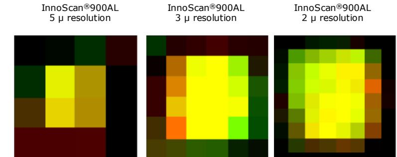
Figure 4b. Zoomed-in image of feature from Circle B in Figure 4a showing increased number of pixels per feature for a 13  $\mu$  diameter feature as resolution increases. Note 4 pixels for 5  $\mu$  resolution image, 16 pixels for 3  $\mu$  image, and 36 pixels for 2  $\mu$  images.
