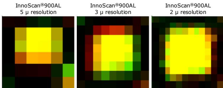
Figure 3b. Zoomed-in image of the upper left feature from Circle A in Figure 3a showing increased number of pixels per feature for a 16  $\mu$  diameter feature as resolution increases. Note 12 pixels for 5  $\mu$  resolution image, 38 pixels for 3  $\mu$  image, and 56 pixels for 2  $\mu$  images.
