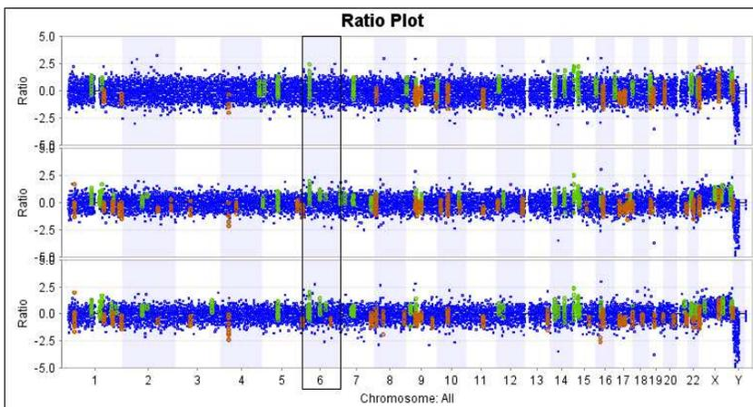
Figure 5. Comparison of ratio plots of the same microarray scanned at 5  $\mu$  (top), 3  $\mu$  (middle) and 2  $\mu$  (bottom) resolution on the InnoScan®900AL. Note, for example, that in chromosome 6 (in box) successively more aberrations (in green or red) were detected at 3  $\mu$  resolution than at 5  $\mu$  resolution; and still more were detected at 2  $\mu$  resolution than at 3  $\mu$  resolution.
