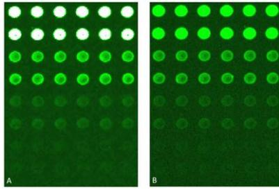
**Figure 2. Dynamic range extension (XDR).** In order to address the issues associated with different protein expression in samples, Innopsys has developed a scan mode to avoid saturation while keeping weak signals. A) RPPA slide scanned in a manual mode; the result image is a 16-bit TIF image with a dynamic range 4 logs. B) The same slide scanned with a XDR scan mode; the image is a 20-bit TIF image with a dynamic range higher than 6 logs.
