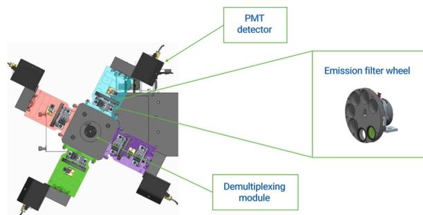
Fig 3. Optical design of the detection ensemble.
