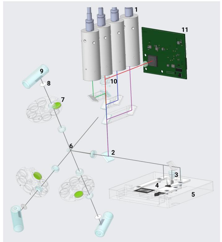
**Fig 7. InnoQuant optical pathway, edited with Creo software.**
