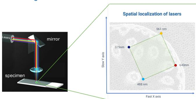
Fig 1. Spatial incidence of excitation lasers on the slide. The four lasers scan the sample simultaneously.
