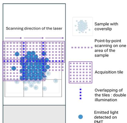
**Fig 4. confocal technology, scan in progress.** The laser spot excites the sample point by point along a line, until the image is complete. The final whole sample full image consists in several overlapped acquisition tiles.
