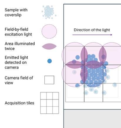
**Fig 5. Widefield technology, acquisition in progress.** The light illuminates the sample field-by-field and the emitted light is detected by a camera. The camera chipset allows the capture of rectangular acquisition tiles.
