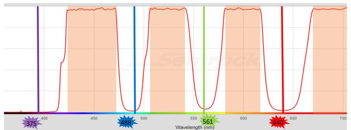
**Fig 8. Dichroic mirror optical features.** Dichroic mirror transmission bandwidth spectrum (red) with excitation wavelengths (vertical continuous lines). Orange regions represent the over 90% transmission bandwidths.
